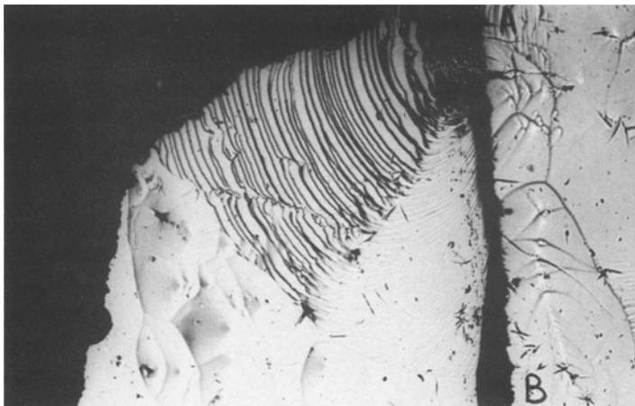
Figure 6 A fissure-like crack AB on the surface of an ErFeO 3 crystal. A growth pyramid having its centre of initiation on the edge of the crack is seen, \times 45 .
